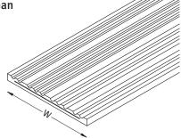
Gantrail flat pad is normally supplied in 12 metre lengths of the widths shown but is also available in lengths and widths to suit customer specification. This may result in longer lead times – Please contact GANTRAIL for guidance.
